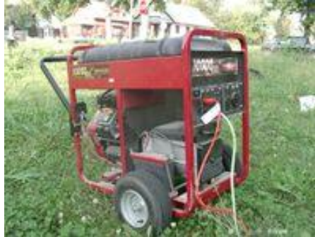
Fig 3.1 Portable generator side view showing gasoline engine.
